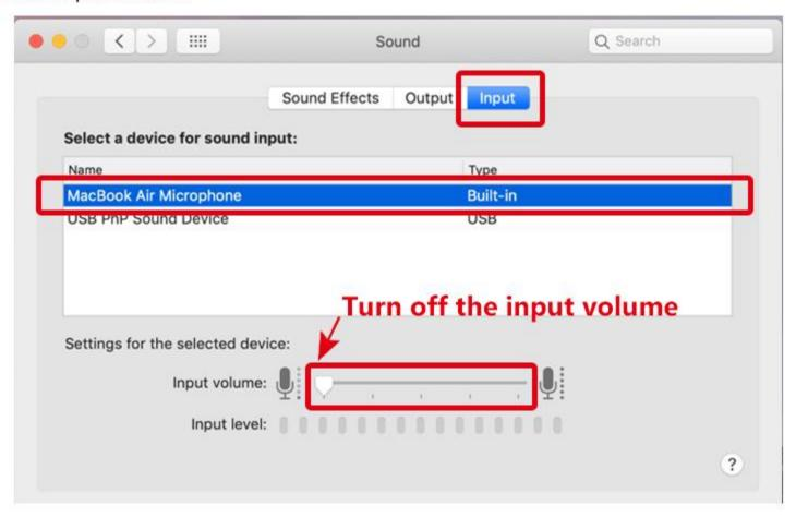
Choose "USB PnP Sound Device", and adjust input volume (general adjustment to the middle).
